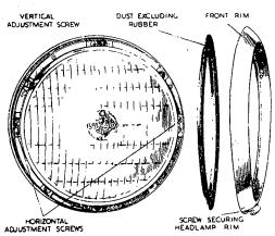
against the tension of the adjustment screw springs and turn it in an anti-clockwise direction until the heads of the screws can be disengaged through the slotted holes in the Light Unit rim. Do not disturb the screws when removing the Light Unit or the Lamp setting will be altered.
