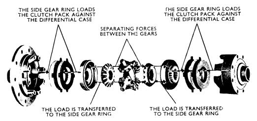
LOADING DUE TO SEPARATING FORCES OF DIFFERENTIAL GEARS
