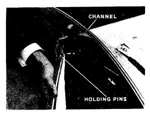
3. Remove the soft top from the pocket provided at rear of seats, holding the metal front section near the centre pins.
