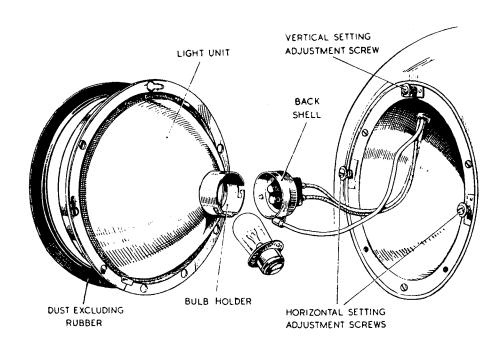
Position the Light Unit so that the heads of the adjusting screws protrude through the slotted holes in the flange, press the unit in and turn in a clockwise direction. Replace the rubber ring so that the thicker inner edge rests in the recess around the Light Unit rim.
