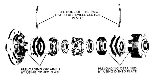
LOADING OF FRICTION CLUTCHES BY BELLEVILLE SPRING
