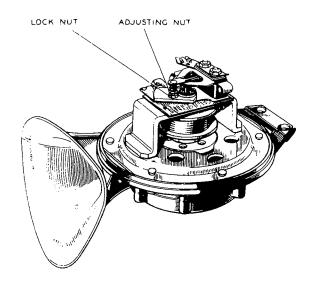
It is also possible that the performance of a horn may be upset by the fixing bolt working loose, or by some component near the horn being loose. If after carrying out the above examination the trouble is not rectified, the horn may need adjustment; but this should not be necessary until the horns have been in service for a long period.
